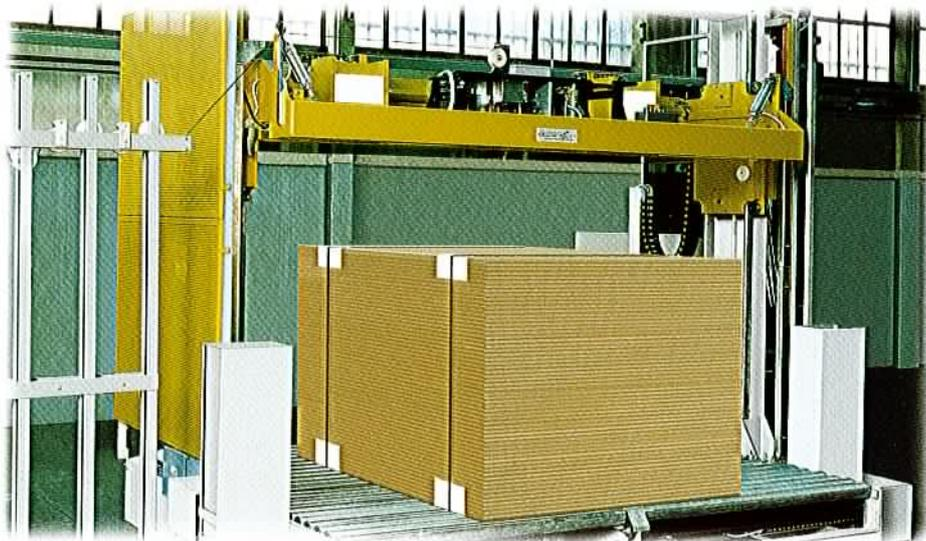
*Designed for strapping bales with automatic feeding of 195x195 mm piled cardboard sheets. It is programmed to perform one or more automatic strappings. The CH type is equipped with 1 head and lower and upper cardboard protections.*
