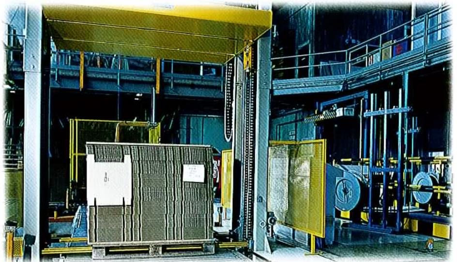
*Designed for strapping pallets or bales with height of 500 to 2,850 mm. It automatically performs one or more strappings.*
