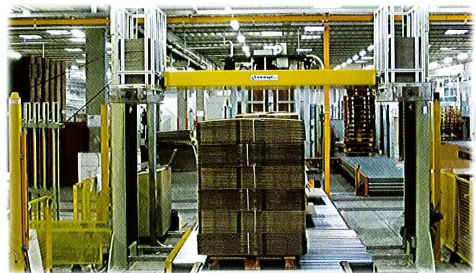
*Designed for strapping pallets or bales with height of 500 to 2,850 mm. It automatically feeds corrugated cardboard protections for ultimate product protection. It automatically performs one or more strappings. PR2MFL type can strap over 100 pallets an hour.*
