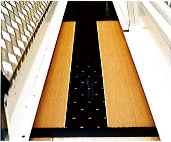
The vacuum transport system guarantees box quality. Sliding, smearing, print register discrepancies and uneven slotting are no longer problems.
