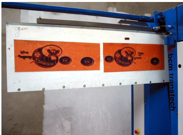
A "dirty" Stereo running into the washing machine
