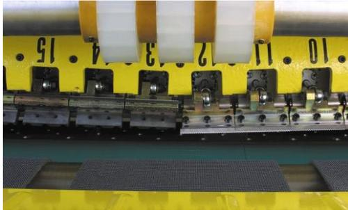
Fosber's patented CONSTANT SYSTEM order allows a true gapless order change on two knife levels through the cut-off knife. The problems of conventional order changes are eliminated by removing the need to sever the web at the rotary shear. This unique order change sequence requires the installation of the CONSTANT SYSTEM Rotary Shear with the Fosber TWIN automatic slitter scorer.
