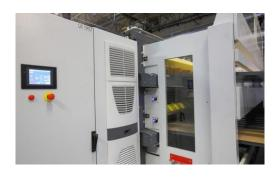
The Master cut-off knife is comprised of three main sections – the infeed delivery section, the cutting section, and the outfeed delivery section.
