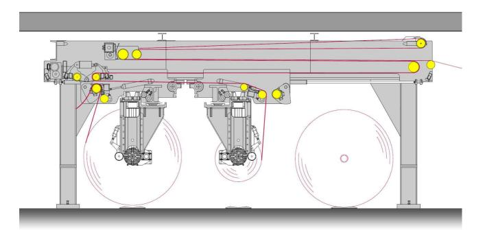
The Link-M3 combined reel stand & splicer group is a unique integrated solution for the optimum running of paper rolls on the corrugator, providing the shortest continuous automatic roll change cycle time available in the industry. Even if the corrugator is located close to a wall, as all reel handling is contained to just one side of the corrugator the Link-M3 roll change cycle time (70% less than conventional systems) is completely unaffected.
