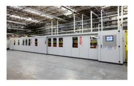
Utilising the most up-to-date technology available today the Express double facer is capable of running the full range of board grades up to 350 mpm, up to a maximum paper width of 2800 mm. Gradual and efficient heat transfer is precisely managed and controlled to achieve and complete an optimum bond whilst maintaining an equal moisture balance according to the running speed and particular board grade being produced.
