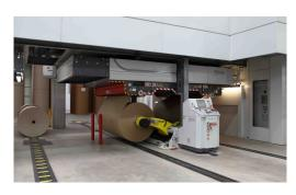
The Link automatic splicer provides the latest automatic splicing technology, integrating precision and reliability through simplistic design. Constructed on a robust support frame to complement bridge integration the Link operates within a range of splicing speeds up to 450 mpm. for the optimum running of paper rolls on the corrugator. It can be associated with our rollstand model Stand M2, available with
