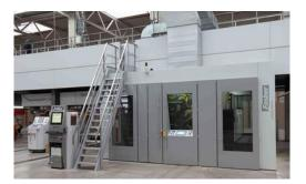
The Smart single facer is a high speed, quick flute change, cassette machine, housed in a very heavy duty, rigid cast iron frame. The mas-
