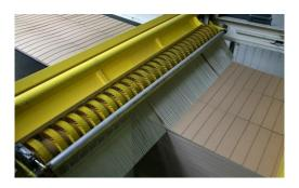
Fosber's latest automatic stacker system, the Terminal, can be configured with one, two or three independent stacker levels. Essentially the Terminal is composed of 4 independently controlled conveyor belt sections, a braking section, a separation section and a downstacker type elevator deck expulsion section.
