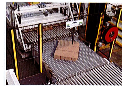
Ball table (patented) Turning of multiple bundles simultaneously
