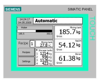
On the left side you will see the local touch screen. When the remote console (PC) is out of order all necessary program tasks can be done on the local screen.
